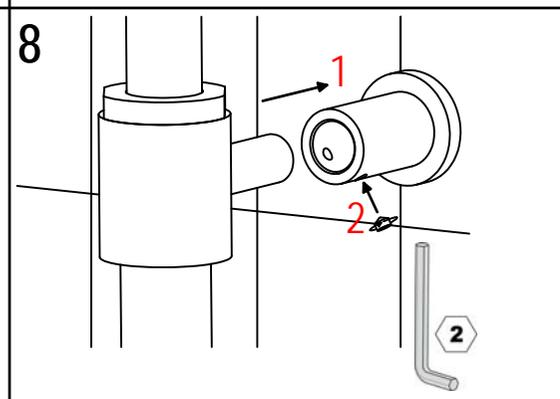
**! SOSTITUZIONE CARTUCCIA / CARTRIDGE REPLACEMENT**
