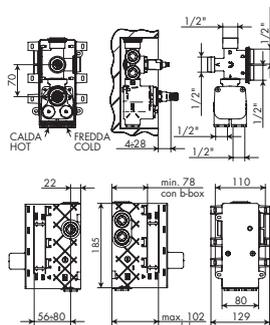
**PARTE INCASSO TERMOSTATICO C/DEVIATORE 4 USCITE 1/2"**
