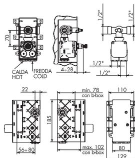
**PARTE INCASSO TERMOSTATICO C/DEVIATORE 2 USCITE 1/2"**
