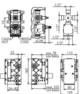
**PARTE INCASSO TERMOSTATICO C/DEVIATORE 3 USCITE 1/2"**
